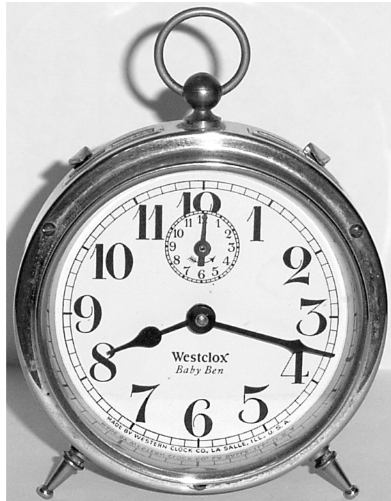
Fig. 16 Style 1 Baby Ben dated January 1929. Note the loop top “X” and ball shaped pendant. (Alarm hand is from a later style clock).
